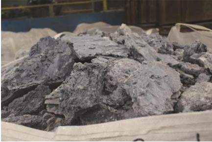
Potassium Aluminium Fluoride (PAF) is a commercial grade fused solid, inorganic salt comprising of a mixture of potassium hexa- and tetrafluoroaluminaes ( $K_3AlF_6$  and  $KAlF_4$ ). The material serves as an alternative to conventional fluoride salts for a variety of applications, a few of which are listed below.
