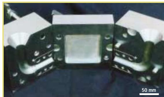
Figure 1 – Photograph showing the three-part steel permanent mould used in the experimental work.
